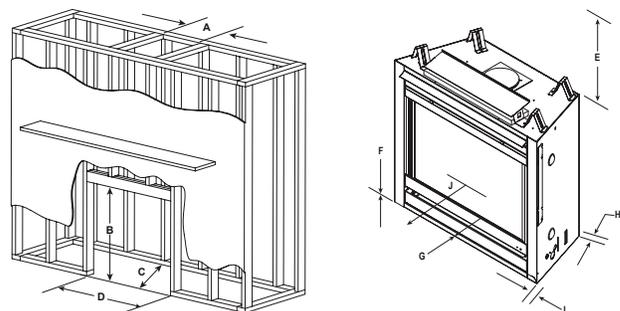
The rough framing dimensions shown represent the distance from stud to stud only and do not take into consideration the addition of drywall. Please refer to installation instructions for complete specifications and drawings when installing this product. Go to [heatilator.com](http://heatilator.com) to download.
